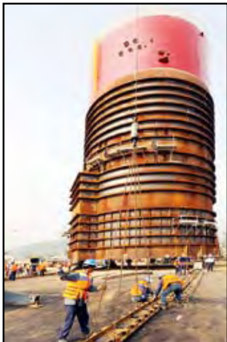
A 670-ton, 45-meter-tall STP cylinder at the APL Norway Peregrino FPSO unit made for Maersk Inc.
